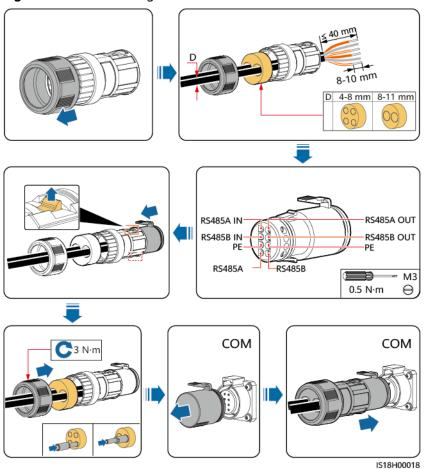
Figure 5-20 Connecting communications cables
