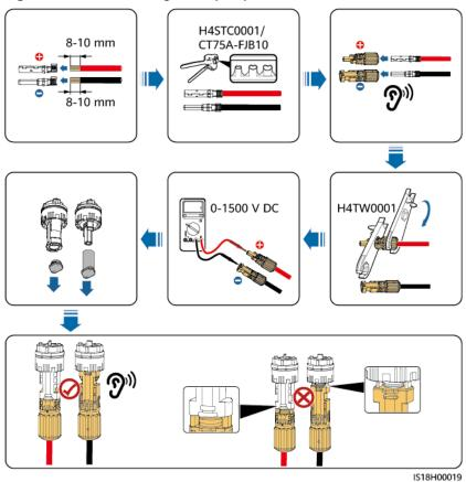
Figure 5-18 Connecting DC input power cables
