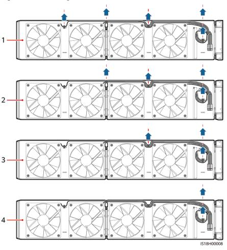
Figure 8-4 Removing cable ties
