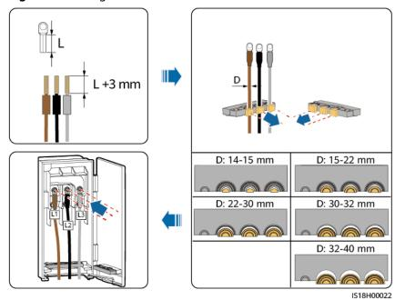
Figure 5-12 Single-core cable connection
