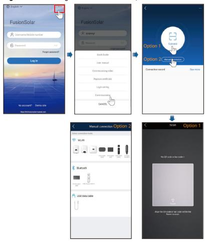
Figure 7-5 Selecting a connection mode (Internet access unavailable)
