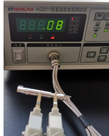
图片 2 LEADER 插针 & TS4 插套 LEADER pin & TS4 socket
