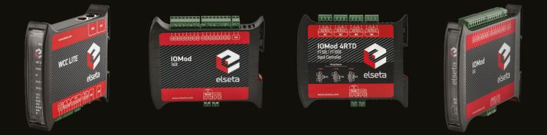
You can combine different input/output modules for system extension. The core **WCC Lite** unit communicates with I/O modules through Modbus (RTU) or IEC60870-5-103 protocol. Adding and configuring each I/O module is almost PlugnPlay.
