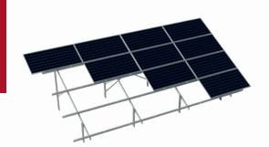
Structure: Two-support, driven into the ground
