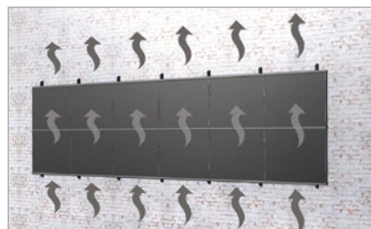
Very good rear ventilation of the modules
