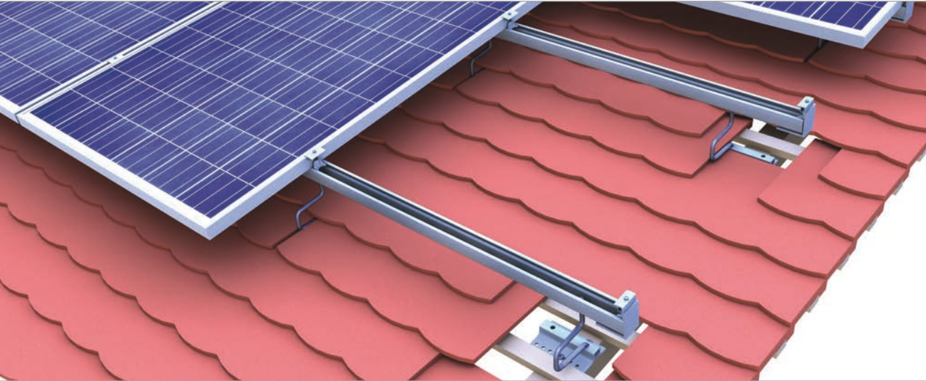
novotegra top-fix – single-rail clamping system on beavertail tile roofing with modules installed in portrait.
