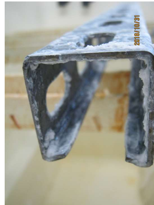
Element after 800h in the salt chamber
