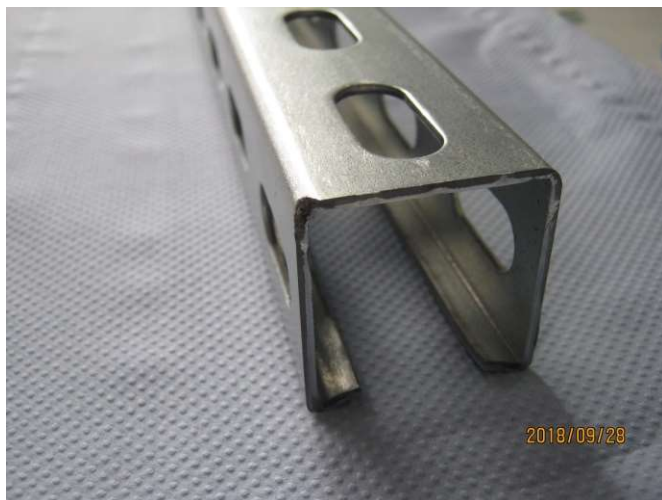
Element before testing in the salt chamber
