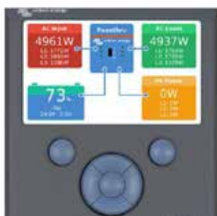
Color Control GX, showing a PV application
